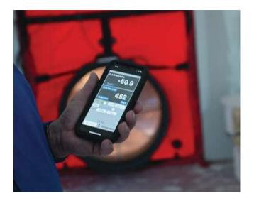
Be aware that blower door air leakage tests are also conducted by creating a pressure difference of 50 pascals between the inside and outside of the structure being tested. The leakage rate is often referred to as air changes per hour at 50 pascals of pressure or ACH50. Properly installed SIP structures regularly achieve leakage rates below 2.0 air changes per hour at a pressure of 50 pascals (ACH50), to as low as 0.3 ACH50 which is below the Passive House standard of 0.6 ACH50.
