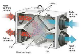
HRV: Heat Recovery Ventilator ERV: Energy Recovery Ventilator
