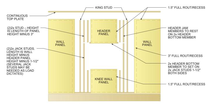
ALL SIP JOINTS SHALL BE AIR SEALED WITH SEALANT AND/OR SIP TAPE. FOLLOW SIP MANUFACTURER'S RECOMMENDATIONS FOR SIP TAPE WIDTHS AND SEALANT PATTERN AND THICKNESSES.
