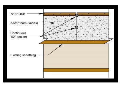
Figure 20. Butt Joint Detail with Sealant
