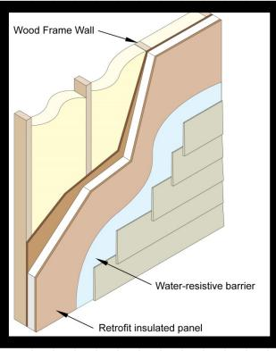
Figure 1. Retrofit Insulated Panel Over Existing Sheathing
