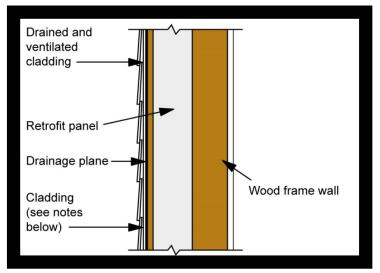
Figure 22. Retrofit Insulated Panel with Rain Screen
