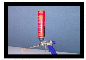
Figure 15.Spray Foam Application Gun
