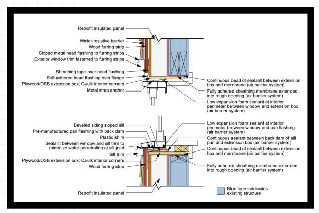
Figure 9. Window Mounted at Exterior Plane
