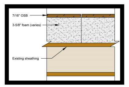
Figure 21. Butt Joint without Sealant
