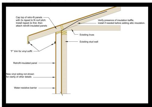
Figure 23. Soffitt Detail for Vinyl Siding
