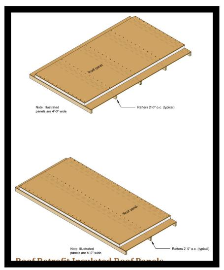
Figure 13. Roof Retrofit Panels Applied to Structural Members
