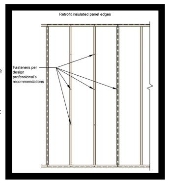
Figure 6. Wall Retrofit Insulated Panels
