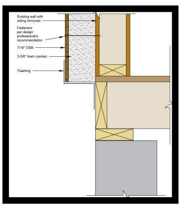
Figure 4. Alternate Retrofit Insulated Panel Rim Joist Detail
