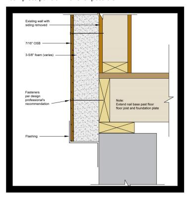
Figure 3. Retrofit Insulated Panel Extended Over Rim Joist
