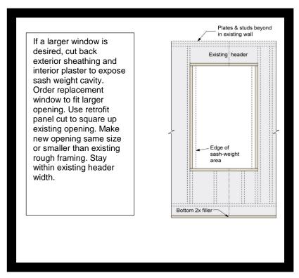
Figure 10. Replacing Sash-Type Windows
