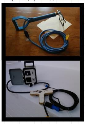
Figure 16. Electric Foam Scoop and Electric
