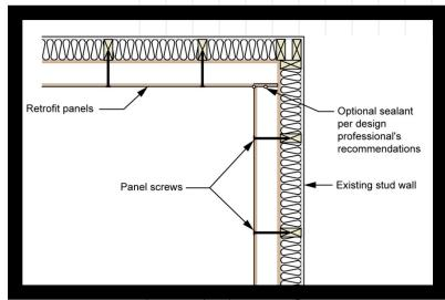
Figure 5. Inside Corner Detail.
