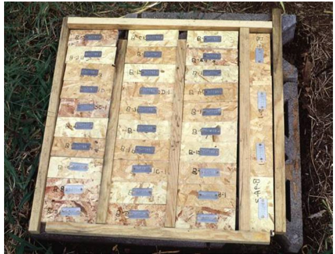
ZB OSB test units placed on top of Formosan Subterranean Termite colony
