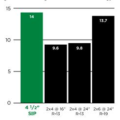
Proven efficiency comes from whole wall R-value calculations for the panelized SIP system, which factor in more than a single material's R-value to include the thermal effects of the entire assembly (including structural members at windows, doors and wall corners).
