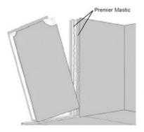
Check the panel dimensions against the floor layout. Apply a 3/8" diameter bead of Premier Mastic along the sides and down the center of the bottom plate. Slide the panel into position. Lift the panel over the bottom plate by using either manpower or mechanical means. After the
