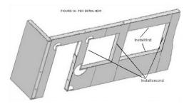
Fur out both sides of the Insul-Beam II with 7/16" sheathing to match the thickness of the panels, keeping the sheathing flush with the top of the top plate.
