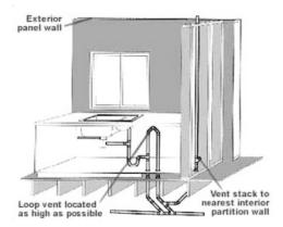
Situations do arise in which it becomes necessary for a builder to consider options for chases in the exterior walls such as a kitchen sink next to a window or washer and dryer unit next to an exterior wall. This situation can be answered through the use of an "island vent" through the floor to the nearest interior wall.
