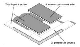
Once the 2' sections are in place, layout the remaining 4' x 8' foam sheets.
