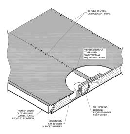
**PANEL TIP >** Stagger your panel placement with two panels on one side of the beam, four panels on the other side, and four back on the first side of the beam. This will help your beam stay straight.
