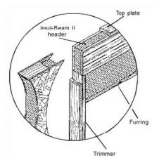
Measure the total depth of the header required and add any sheathing or plating to the top or bottom of the header to achieve this dimension. Measure the maximum length the header can be and cut the header 1/8" short of this, taking care to avoid the nails in the Insul-Beam II as you cut.
