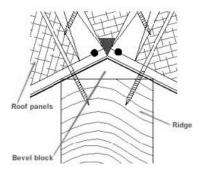
Cut a bevel block out of dimensional lumber to the same pitch as the roof and fasten the full length of the ridge. The roof panel must bear at least  $1 \ 1/2$ " on the beveled block. Next, tack SIP Tape that is 18" wide on top of the ridge beam. (Be sure that the release paper is facing up towards the underside of the roof panels.)
