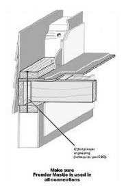
Another option: Once the top plate is in, you may now also hang joists directly from the wall panel. Use a joist hanger with a nailable top flange. The flange should bear at least 1.5" (2" is best) on to the top plate. Nail the top flange following the fastening schedule specified by the engineer.
