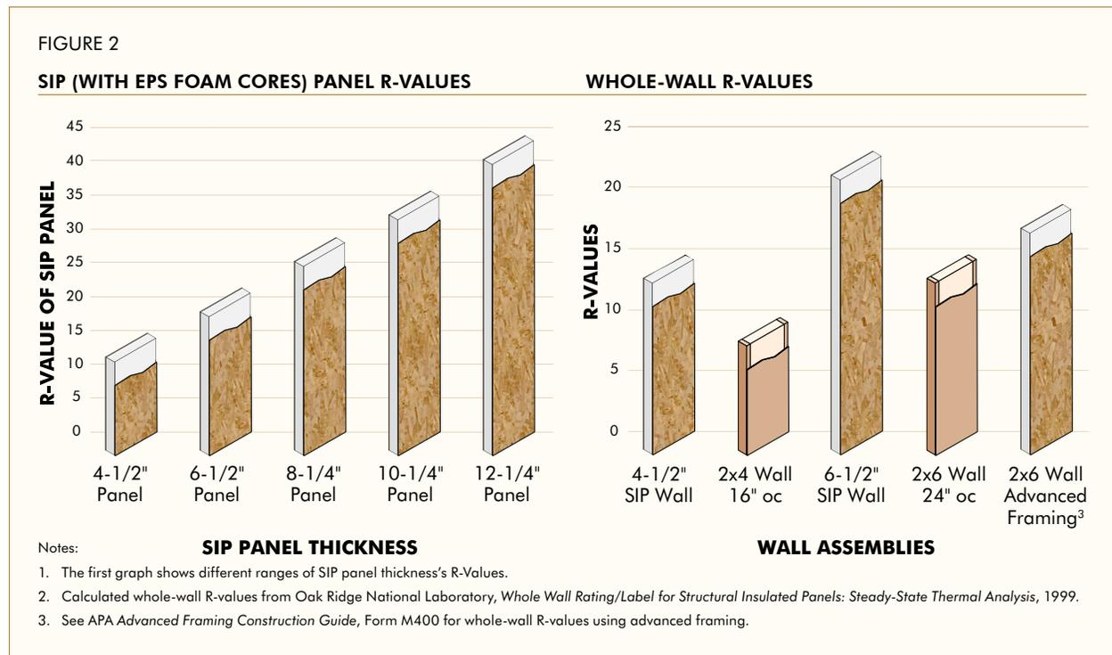
When working with panels as large as 8 x 24 feet, there are significantly fewer joints that require sealing. SIPs establish a whole-house air barrier simply and effectively. Studies at the U.S. Department of Energy's (DOE) Oak Ridge National Laboratory (ORNL) show a SIP room to have 90 percent less leakage than its stick-framed counterpart.<sup>a</sup>
