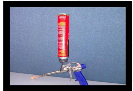
Figure 15. Spray Foam Application Gun
