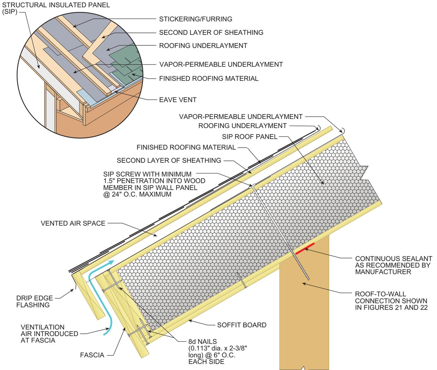
ALL SIP JOINTS SHALL BE AIR SEALED WITH SEALANT AND/OR SIP TAPE. FOLLOW SIP MANUFACTURER'S RECOMMENDATIONS FOR SIP TAPE WIDTHS AND SEALANT PATTERN AND THICKNESSES.
